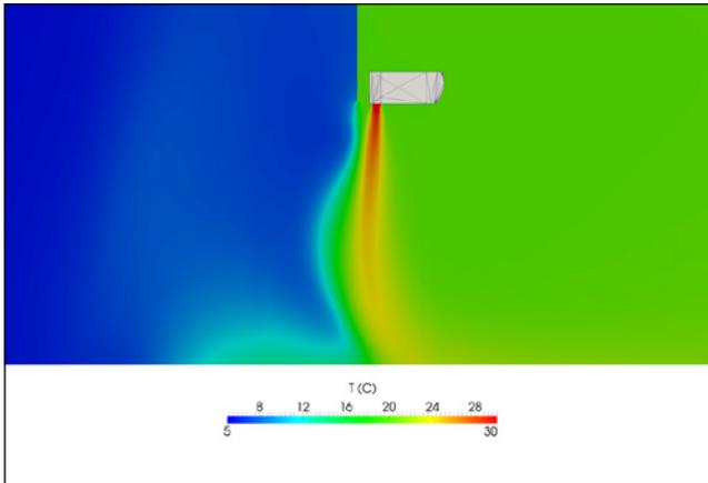
A thermographic image proves the clear separation of warm and cold air.
